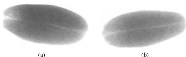
Fig. 1. Logarithmic subtracted dual energy X-ray images of (a) vitreous and (b) non-vitreous kernels.
