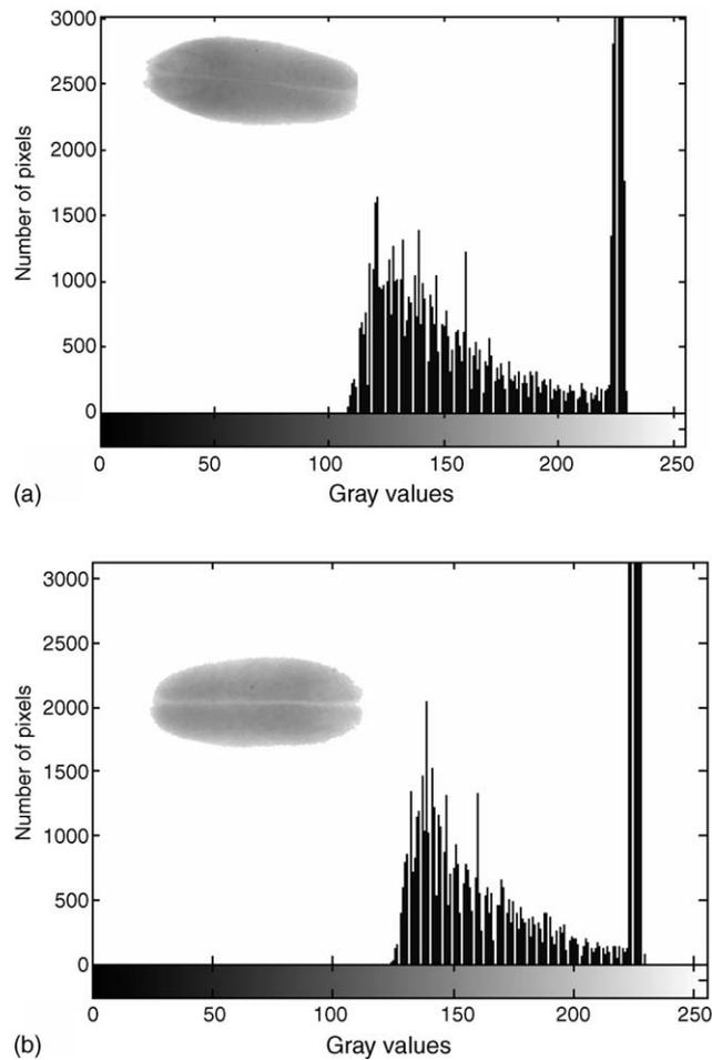
Fig. 3. Histograms of durum wheat kernel X-ray images (a) vitreous (b) non-vitreous (0 represents black and 255 represents white in the X-axes).
