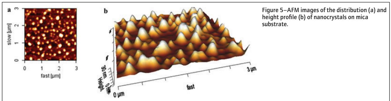
Figure 5—AFM images of the distribution (a) and height profile (b) of nanocrystals on mica substrate.
