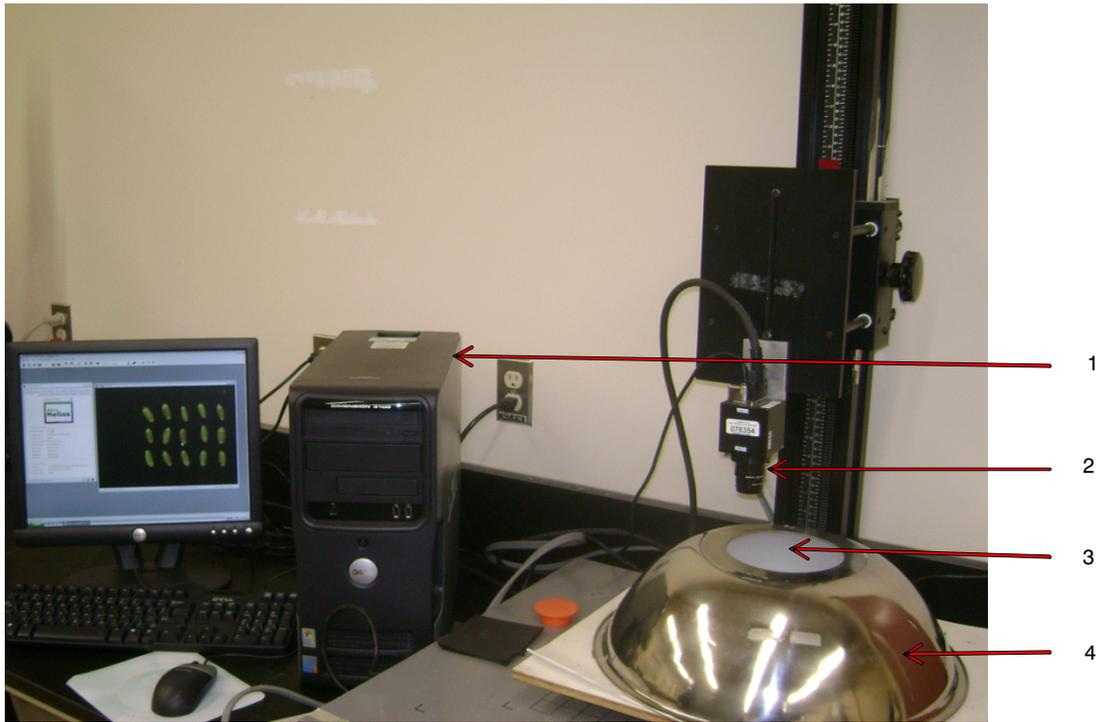
1 - Processor; 2 - Digital camera; 3 - Illumination chamber; 4 - Light diffuser
