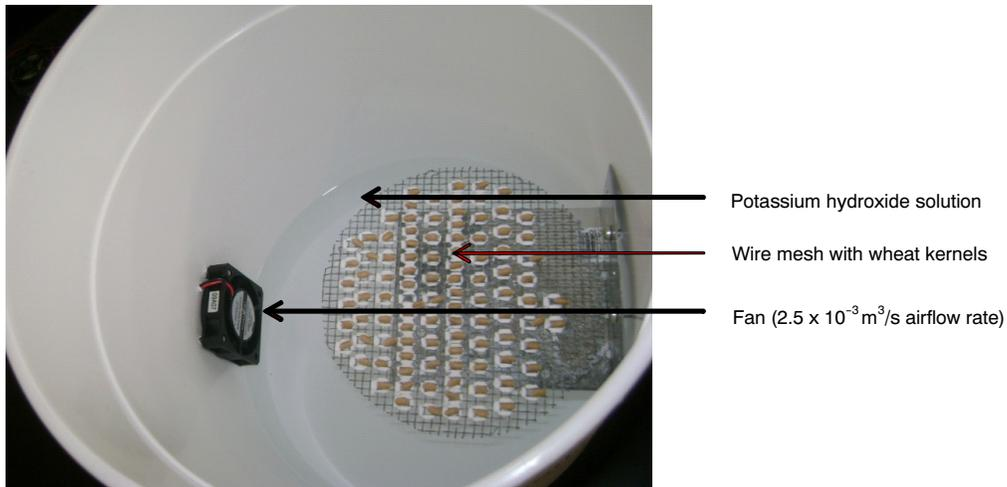
Figure 1. Machine vision system and grain conditioning set up.
